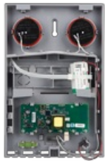
JA-163A-BASE-RB - bottom part with electronics
