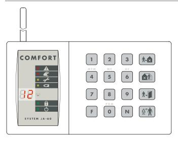
The JA-60F is an optional wireless keypad for the JA-60 or JA-65 series wireless control panel. It can operate the system in exactly the same way as the built-in keypad on the control panel and as the hard wired bus system keypad, JA-60E. The LED indicators, display and built-in buzzer indicate the alarm system's status.
