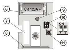
DIP switch 2 The DEL (OFF) position provides entrance & exit delays for detectors installed in a building entrance. The INS (ON) position allows the detector to instantly trigger alarm activation if the control panel is armed. This setting only has an effect if the detector has a natural reaction assigned to it in the Oasis control panel. It also has no effect when used with a UC-8x or AC-8x receiver.
