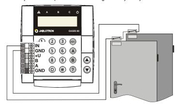
An example of door detector wiring
