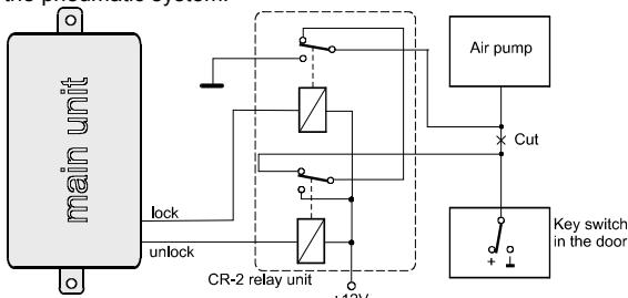
**Simplified additional installation of central locking system:** When manual operation of the whole system from the driver's door is not requested, you can use the following easy solution. Install two-wires actuator (recommended type CM-2) to each door of your car. Connect them as shown in the following diagram. Program duration of Accent output pulses 0.3 seconds. This way all actuators are operated with the remote control.
