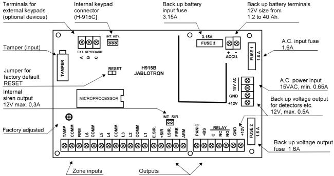
**+BS** - this terminal is for connection with an outdoor back up siren. There is a positive potential supplied by this terminal when the alarm output relay is not switched on.
