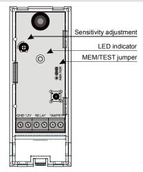
The **Vivo** is designed for indoor applications. It should be mounted on a flat wall. The unit must have an unobstructed view of the protected glass (in the case of heavy curtains, mount the detector on the window frame behind the curtains). Do not place the detector close to any apparatuses that can generate air pressure changes, low frequency noise or vibrations.
