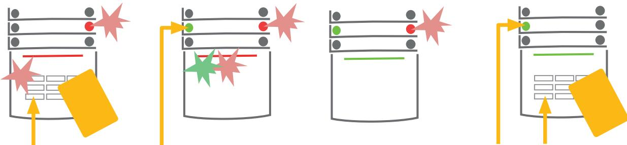
1. Tast inn en kode eller bruk kort/brikke. Press the left segment button of the section where the alarm has been triggered.
