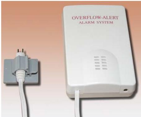
The LD-63HS overflow alarm detector can be used in bathrooms, basements etc., where water detection is required. It is powered locally from alkaline batteries. In case of detection of water leakage a built-in siren goes off. In the same time the normally opened contact of the output relay can trigger an alarm system. Steam or small water droplets won't trigger alarm.
