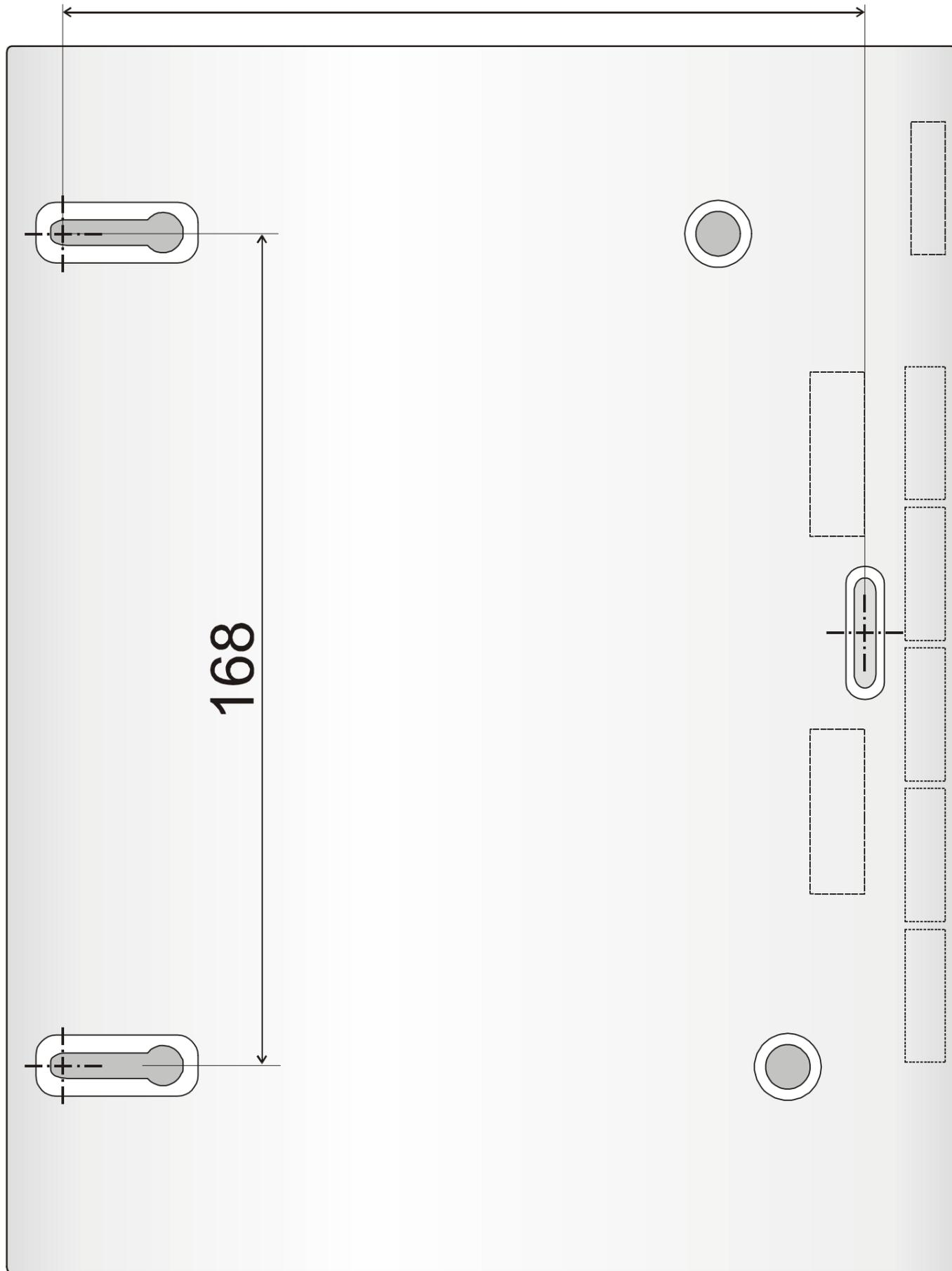
Control panel drilling plan
