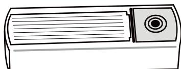
The button should be protected from rain (it is supplied with a plastic roof).
