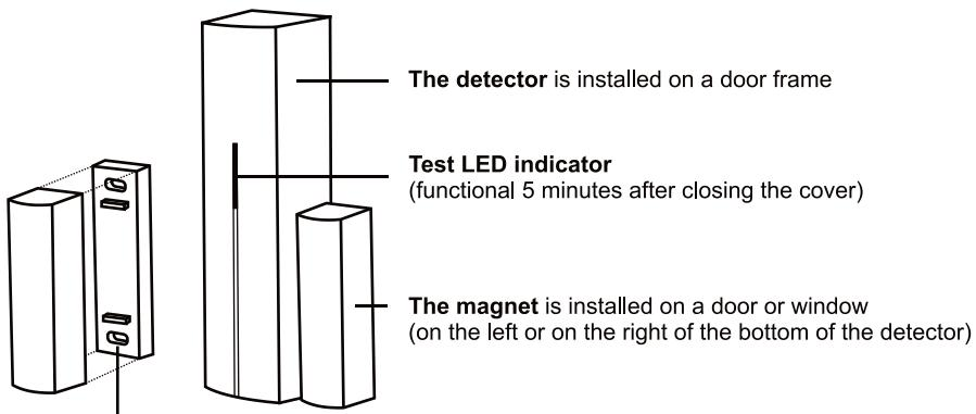
**Magnet pads** (use when installing on a metal surface, they protect the magnetic field from a "short circuit")
