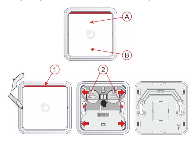
**A**, **B** – buttons; 1 - LED; 2 - holes for fixing screws;
