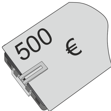
Fig. 2: panic button equipped with a banknote holder
