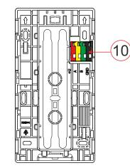
Figure 3 – mounting pad: 10 – BUS terminal
