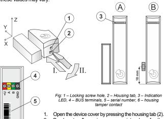
Break out a flange in an appropriate place for the installation, thread a cable through and install the detector onto the chosen location.
