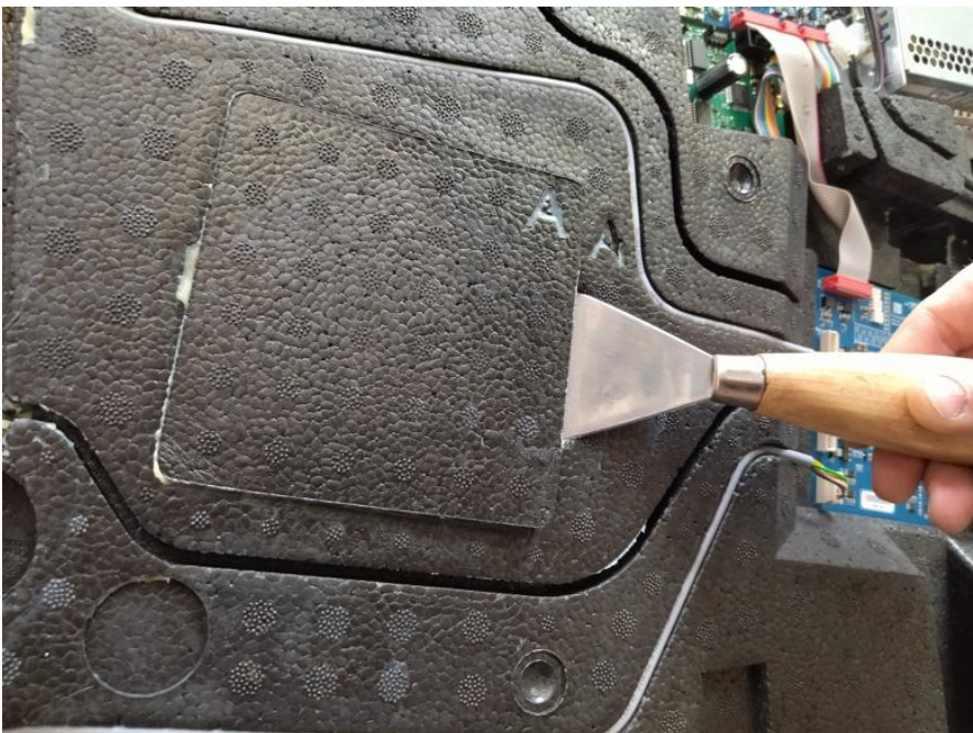
Figure 1 - Inspection plugs removal with spatula
