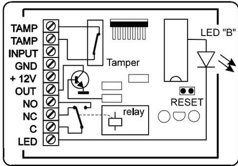
**OUT** terminal is the negative switched transistor output (max. 0.3A/24V). This transistor switches to the GND in the panic condition (PULSE or LATCH mode). In the CONTROL PANEL mode it can be programmed as either a panic output, a pre-alarm output, an alarm memory output or an arm condition output.
