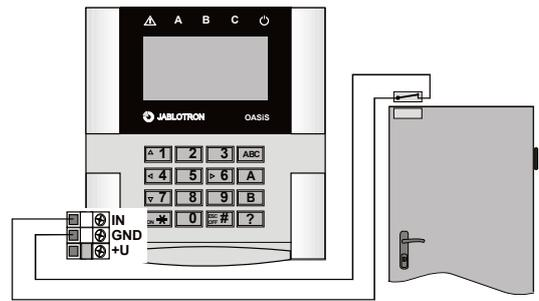
**Note:** The lifetime of the battery is reduced proportionally to how frequently the door detector is triggered and how often and how long the keypad is battery-powered.
