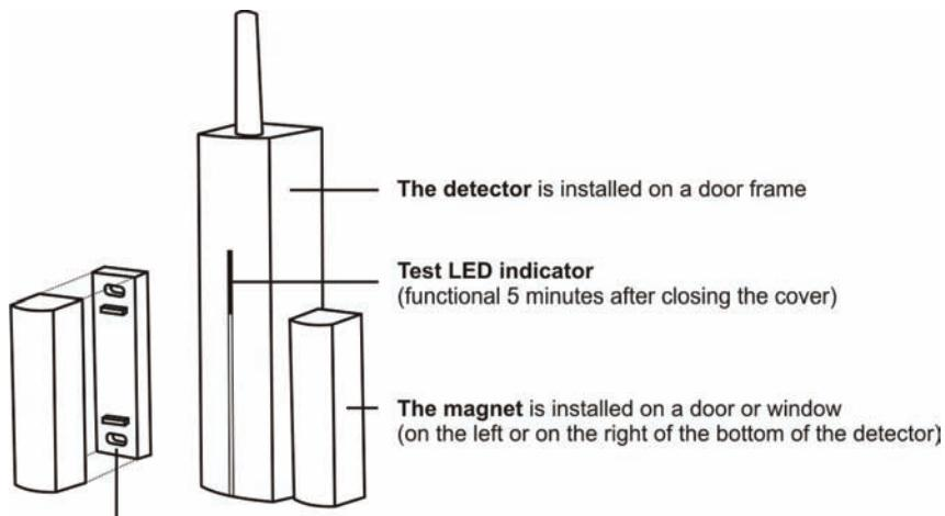
**Magnet pads** (use when installing on a metal surface, they protect the magnetic field from a "short circuit")
