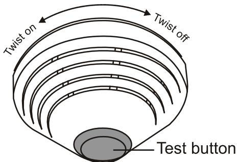
The detector reports fire hazards. It is activated by the presence of smoke or an abnormal temperature increase. Besides sending a report to the system, it also triggers its own siren during an alarm.
