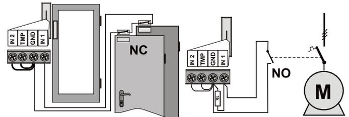
Wiring example for NC ... and NO contacts
