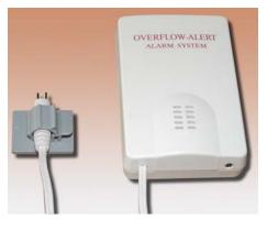
The LD-63HS overflow alarm detector can be used in bathrooms, basements etc., where water detection is required. It is powered locally from alkaline batteries. In case of detection of water leakage a built-in siren goes off. In the same time the normally opened contact of the output relay can trigger an alarm system. Steam or small water droplets won't trigger alarm.
