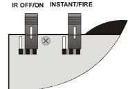
setting is suitable especially for location where the common usage of some appliance (e.g. fire place) may cause a presence of the smoke.
