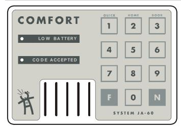
This keypad is an optional part of JA-60 wireless alarm system. It can operate the system similar to the built-in keypad on the control panel. Multiple JA-60D keypads and RC-11 remote controllers can be used with a control panel (max. 8 totally). The keypad has a built in tamper sensor and it also checks the number of attempts to enter an access code (5 unsuccessful attempts will trigger a tamper alarm).
