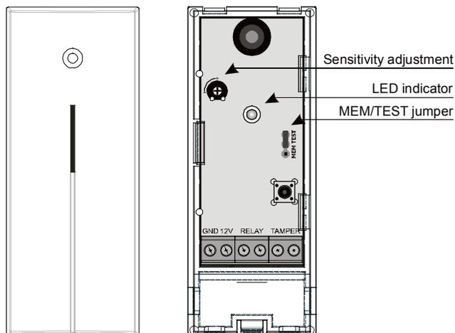
The **Vivo** is designed for indoor applications. It should be mounted on a flat wall. The unit must have an unobstructed view of the protected glass (in the case of heavy curtains, mount the detector on the window frame behind the curtains). Do not place the detector close to any apparatuses that can generate air pressure changes, low frequency noise or vibrations.
