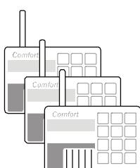
A maximum of eight JA-60D keypads can be enrolled into a single UC-216's memory. The UC-216's outputs will react to all enrolled keypads. For example if any enrolled keypad has an open cover, the UC-216's Y relay will activate.
