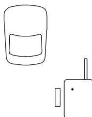
A maximum of eight JA-60 detectors can be enrolled into a single UC-216's memory. The UC-216's outputs will react to all enrolled detectors. For example if any enrolled detector has an opened cover, the UC-216's Y relay will be activated.
