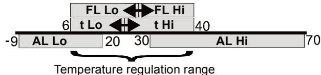
**Temperature accuracy adjustment:** The thermostat allows you to configure the hysteresis – the accuracy to which the temperature is regulated. The setting is done via the **SPAN** item in the adjustment menu (proceed the same way as with the threshold parameters mentioned above). Turning the knob lets you select one of the following accuracy ranges: ±0.1°C, ±0.2°C or ±0.5°C (the factory default setting is ±0.2°C).
