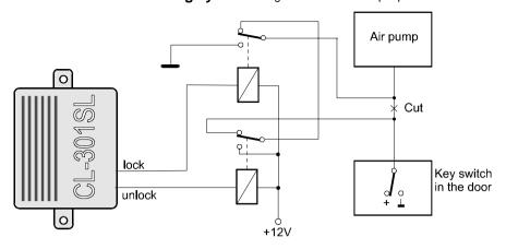
Simplified additional installation of central locking system: When manual operation of the whole system from the driver's door is not requested, you can use the following leasy solution. Install twowires actuator (recommended type CM-2) to each door of your car. Connect them as shown in the following diagram. Program duration of CL-301SL output pulses 0.3 seconds. This way all actuators are operated with the remote control.
