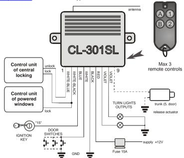
**Installation:** Examine the central locking system of your car and identify the necessary signals of the car wire harness at first. Disconnect the battery before starting the installation. Keep in mind that if your car has memory functions, they may be erased if you disconnect the battery. Refer to the car owners' manual before disconnecting the battery. The lock signal can also be used for automatic closing of powered windows.
