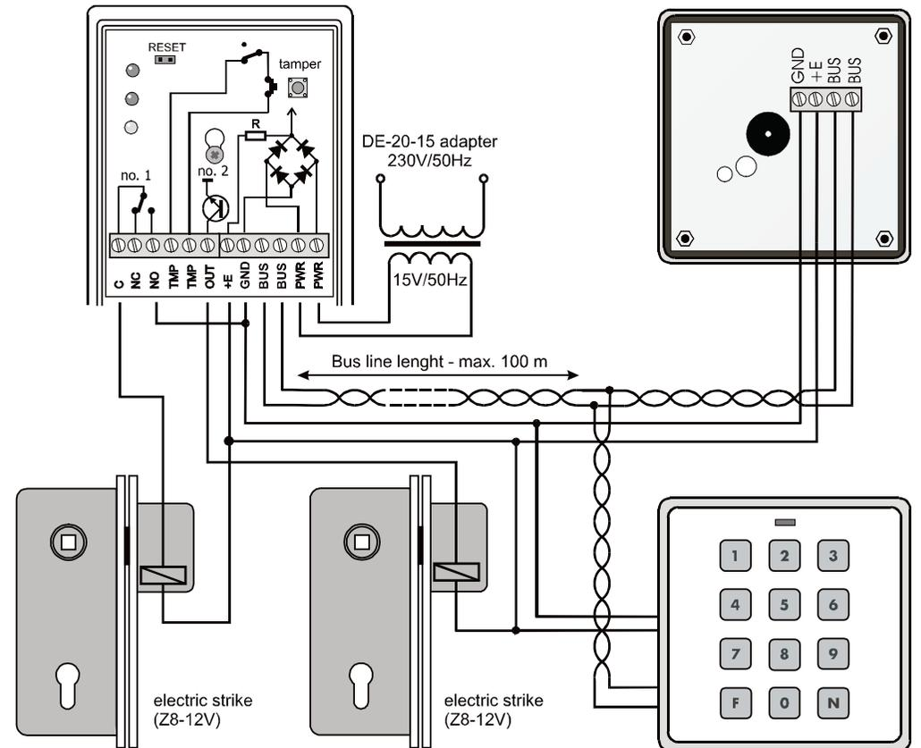
Example two doors access control. AC or DC power supply may be used. Pulse length on outputs N.1 and N.2 should be set to 1 – 5 sec. (depending on the type of electric lock). Garage gates, parking bars etc. can be controlled in a similar way.
