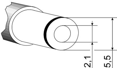
fig. 1 - output connector (all in mm)
